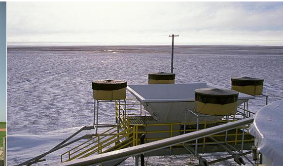
Radar wind profiler
