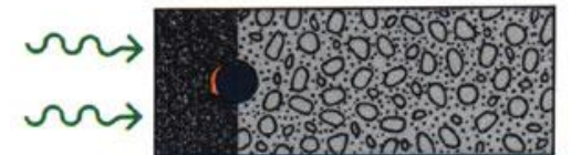
2. CO 2 penetration = carbonization; alkalinity below pH 9
