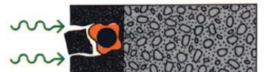
4. Rust formation causes cracks.
