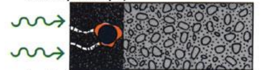
3. Penetration of water and oxygen causes the steel reinforcement to rust after 5 to 20 years.
