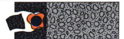
5. Rust expansion causes concrete to crumble away.
