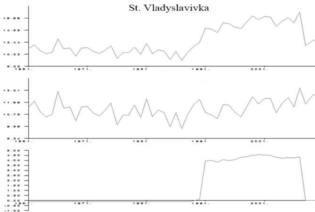
Fig. 2. Example of inhomogeneity in air temperature data: top image - time series before homogenization process, the middle image - time series after homogenization process, bottom image - inhomogeneity
