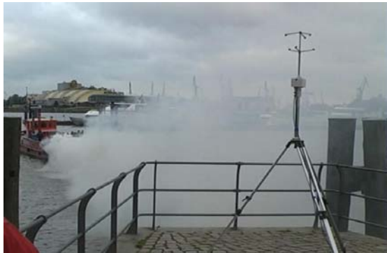
Figure 3. Second campaign at June 19, 2011: (a) Picture from the highly meandering smoke plume and from the ultra sonic anemometer located at 'Kehrwiederspitze'. (b) Wind velocity versus time trace measured simultaneously at 2 different stations during the intensive operation period
