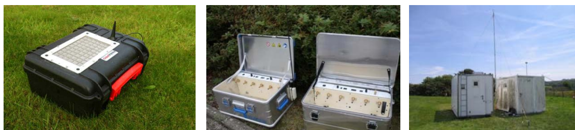
Figure 2. Beta counting proportional counter (Berthold-LB123) (left), air sampler VEGA (middle), and 6-m sonic anemometer for wind measurement (right).
