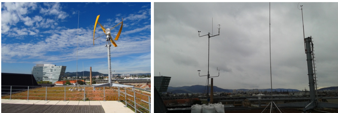
Figure 1. Picture of the SWT (left) and one of the masts with ultrasonics in 3m and 6m above roof level and a sonic at 9m above roof level for site calibration at the SWT mast (right) on the top of the roof of the Energy Base building in the northern part of Vienna.
