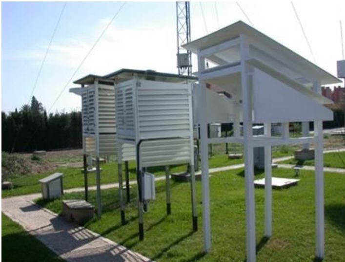
A Montsouri screen (right) and two Stevenson screens (left) used in the SCREEN Project
