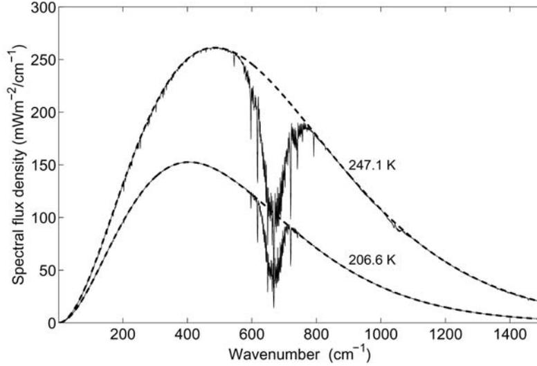
*Fig. 15.* LBL simulations of the spectral flux densities for a warm and a cold standard Martian atmospheric profile. The thin solid line is the spectral  $OLR$  and the thick dashed line is the blackbody function at the indicated surface temperatures.
