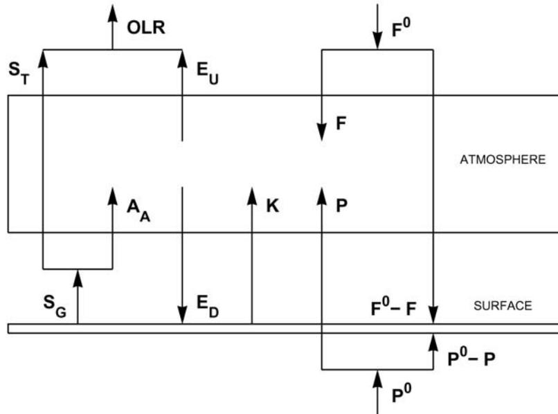
*Fig. 1.* Radiative flux components in a semi-transparent clear planetary atmosphere. Short wave downward:  $F^0$  and  $F$ ; long wave downward:  $E_D$ ; long wave upward:  $OLR$ ,  $E_U$ ,  $S_T$ ,  $A_A$ , and  $S_G$ ; non-radiative origin:  $K$ ,  $P^0$  and  $P$ .
