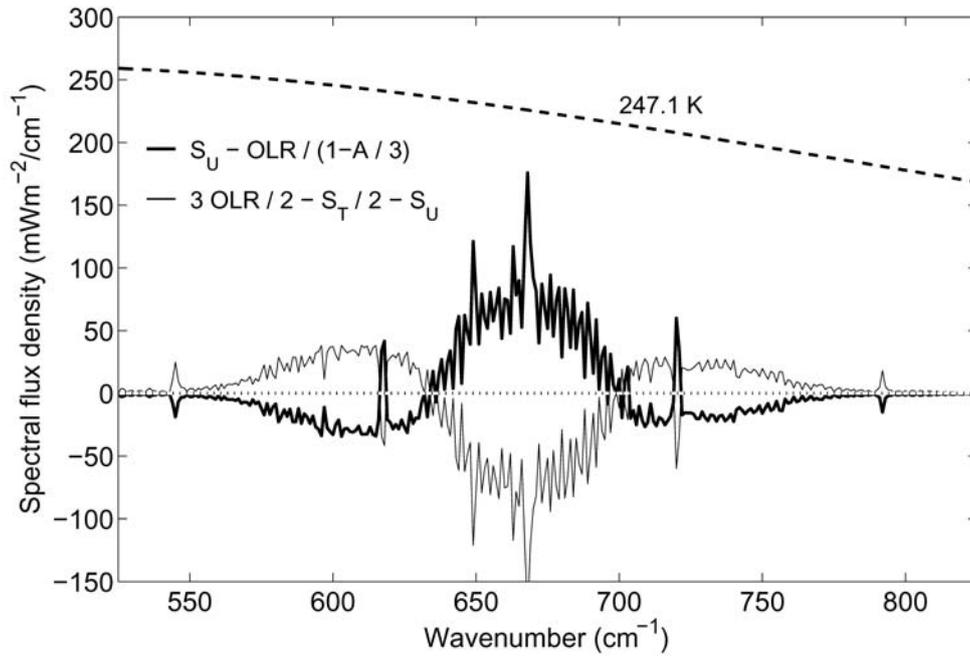
Fig. 18. Spectral flux differences in the  $15 \mu\text{m}$   $\text{CO}_2$  band. The dotted line represents the averaged differences over the  $1\text{--}3490 \text{ cm}^{-1}$  spectral range for both curves. The dashed line is the spectral blackbody radiation at the indicated surface temperature. The spectral differences are compensated over a relatively narrow wavenumber interval around the band center.
