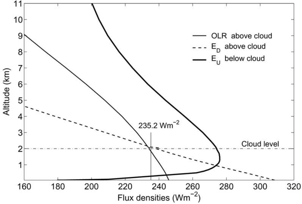
Fig. 6. Cloudy simulation results using the global average temperature and water vapor profiles. For the  $OLR$  and  $E_D$  curves the altitude is the cloud-top level. For the  $E_U$  curve the altitude is the level of the cloud-bottom. Simulations were performed at eleven cloud levels between the 0 and 11 km altitudes. The gray vertical line is the all-sky  $OLR^A$ .
