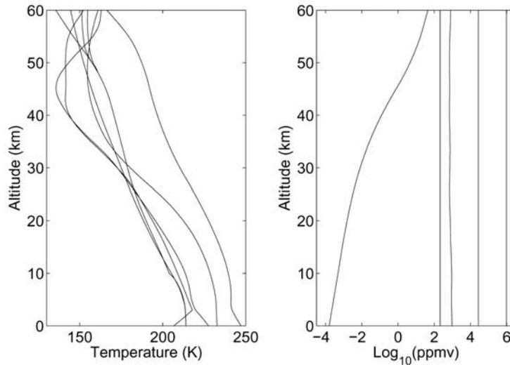
*Fig. 14.* Martian standard temperature and volume mixing ratio profiles. In the right plot the absorbers are (from left to right): O<sub>3</sub>, H<sub>2</sub>O, CO, N<sub>2</sub>, and CO<sub>2</sub>.
