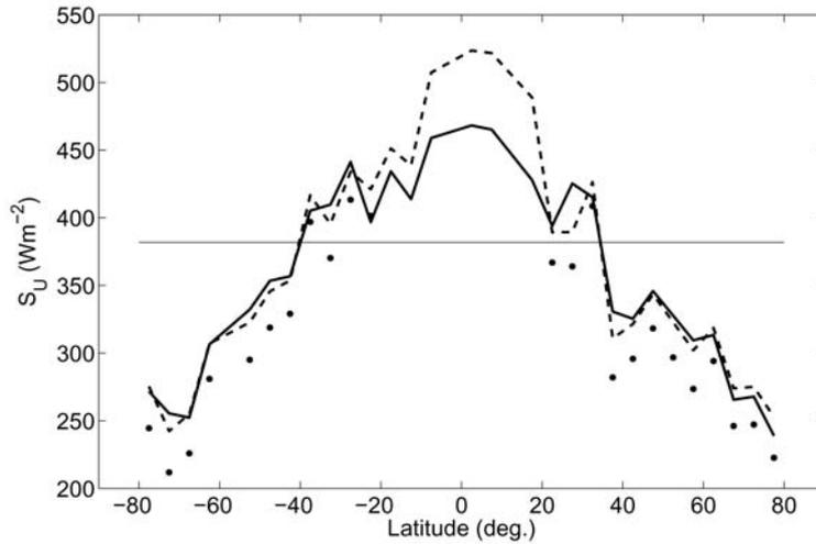
Fig. 12. Meridional distributions of the zonal mean surface upward flux densities. Thick solid line is the observed all sky  $S_U$ . Dashed line is the required  $S_U$  to satisfy the  $S_U = OLR/f$  equation. Thin solid horizontal line is the global average. Dots represent the semi-infinite approximation of  $S_U = OLR(1 + \bar{\tau}_A)/2$  for higher latitudes.
