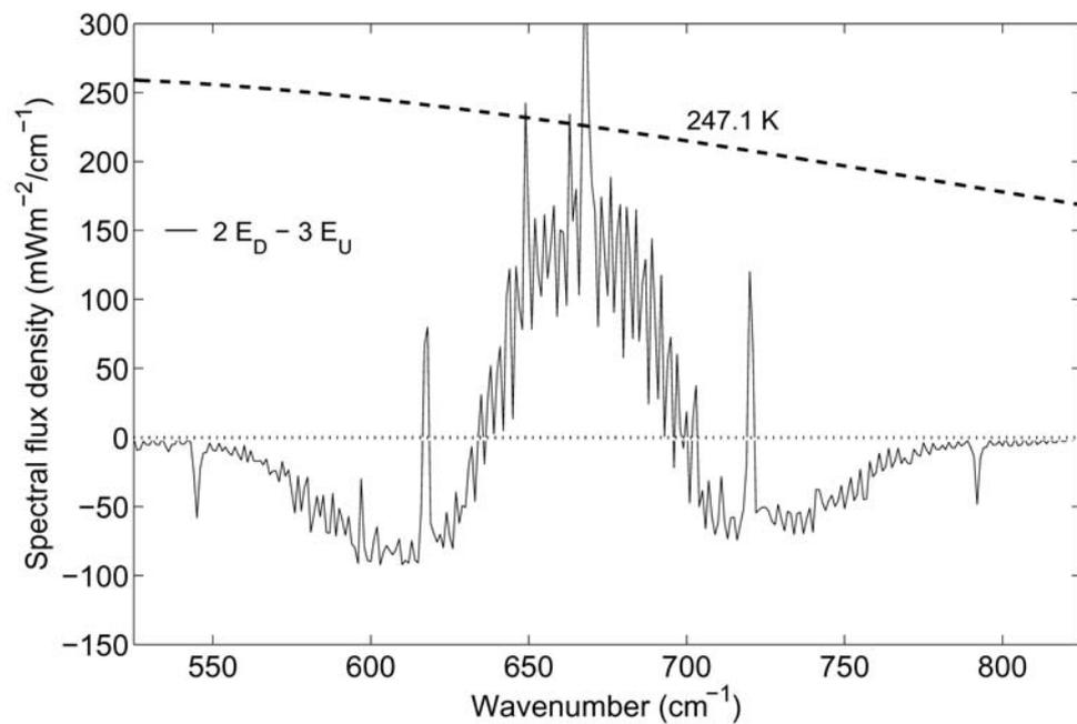
Fig. 19. Spectral differences in the  $2E_D$  and  $3E_U$  flux densities. The dotted line represents the averaged differences over the  $1\text{--}3490 \text{ cm}^{-1}$  spectral range. The dashed line is the spectral blackbody function at the indicated surface temperature. The spectral differences are largely compensated over the extent of the  $15 \mu\text{m}$   $\text{CO}_2$  band.
