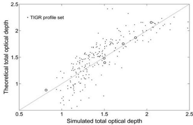
*Fig. 4.* Comparisons of the theoretical and simulated total flux optical depths. The inner four circles were computed for global and zonal mean temperature profiles, the leftmost circle were computed for an extremely cold arctic profile, the rightmost circle represents a mid-latitude summer profile. The dots show the results of 228 LBL simulations. The scatter of the dots are due to the fact that the temperature profiles were not in perfect radiative equilibrium.
