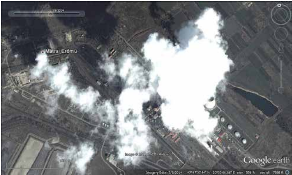
Fig. 3. First type of plume merge in the Mátra Power Plant, Hungary.
