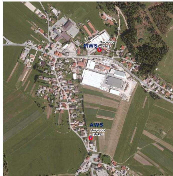
Nova vas on the Bloke plateau (400 meters AWS to MWS): frequent strong nocturnal temperature inversion , different obstacles and difference between thermometer screens
