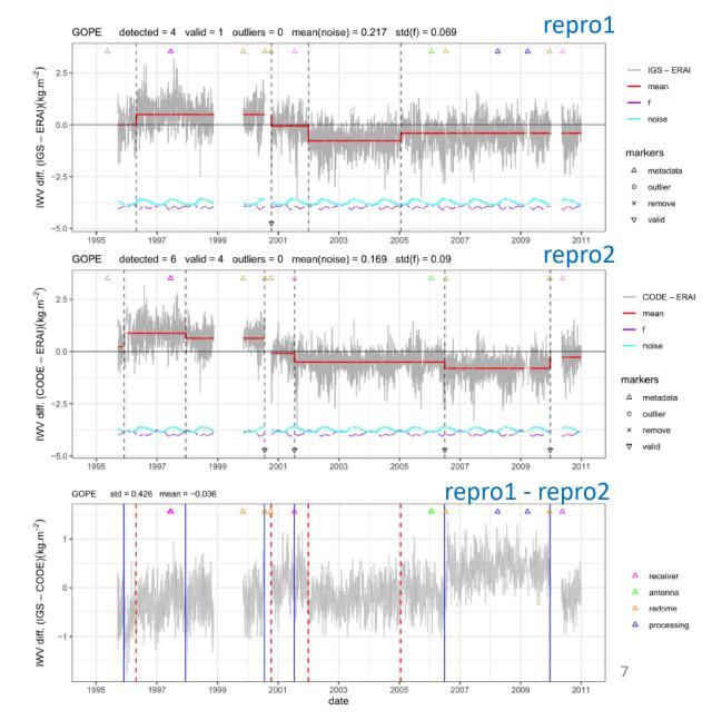
bias between GNSS data sets due to different ant.+rad. models
