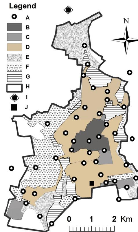
*Fig. 2.* UHI measurement sites (A) and urban morphological types in Beregszász (Berehove): **B**—historical town center with 3–5 storied buildings, **C**— 5–8 storied apartment houses, **D**—1-2 storied detached houses, **E**—open low-rise built-up area, **F**—industrial area, **G**—green areas inside the town, **H**—border of the study area, **I**—rural measurement site (reference point), **J**—weather station.
